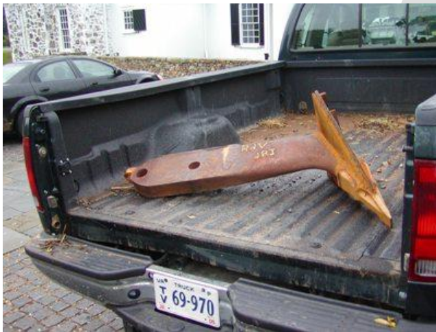
Winged plow for on vine row ripping helps soil and vine uniformity
