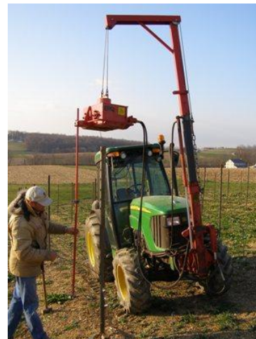
Using a vibrator to install metal line stakes
