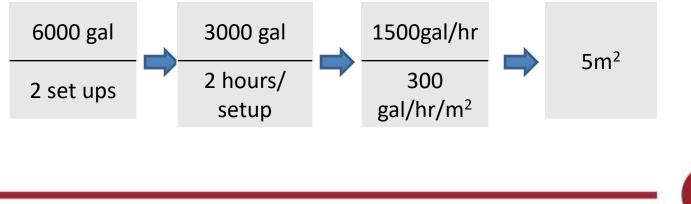
A 5m<sup>2</sup> filter should allow for 6,000 gallons to be filtered in 7 hours including setup/breakdown
